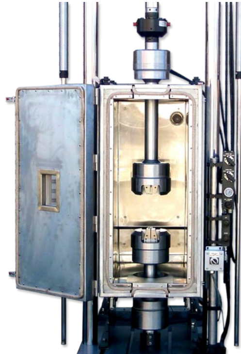
Grip assemblies in load-frame mounted high-temperature test chamber.
