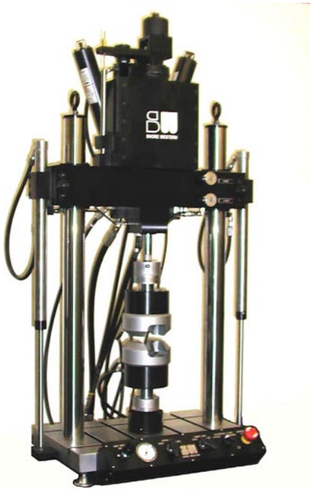
Grips mounted in load frame.
